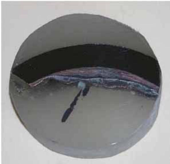
1. Alternating copper metal and iron oxide layers on boiler tube illustrate how corrosion can release copper into the steam circuit of a boiler or into the cooling water from a condenser. Courtesy: Gary Hoffman, "Chemical Cleaning of Natural Circulation Boilers: The Good, the Bad, & the Ugly" (Southwest Chemistry Workshop, Scottsdale, Ariz., July 2005)
