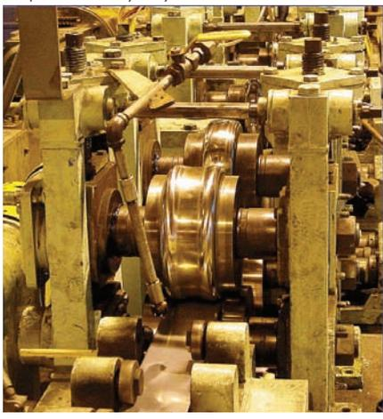
**4. By the numbers.** Forming a round tube from flat stock requires several gradual and precision rolling operations. *Source: Plymouth Tube Co.*
