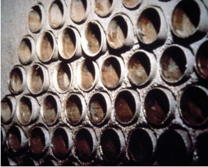
Figure 1. Galvanic attack of a carbon steel tubesheet in contact with stainless steel tubes in high conductivity water (courtesy of Plastocor)
