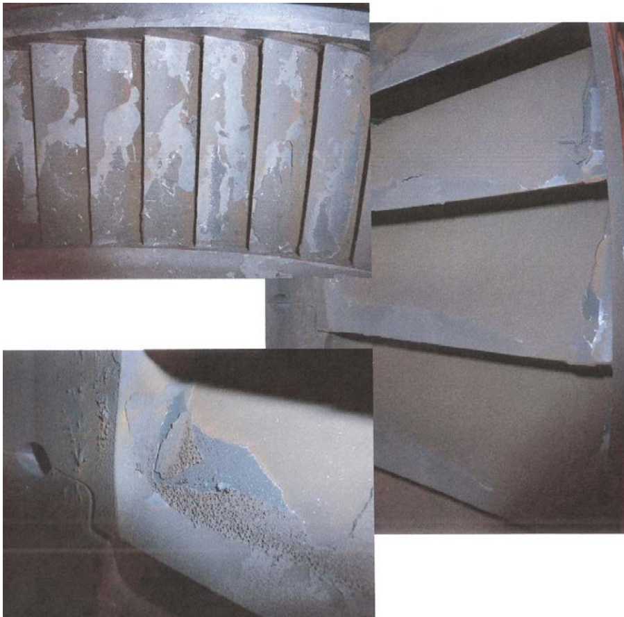
Figure 2. Examples of copper deposits on high pressure steam turbine blades, Source – Elise Ring, API PowerChem 2010 Conference, Caloundra, Australia, May 2010
