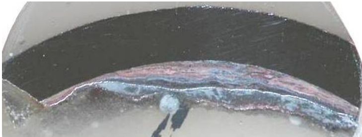
Figure 1. Alternating layers of deposited copper metal and magnetite on a boiler tube. Courtesy of Gary Hoffmann of Pacificorp.
