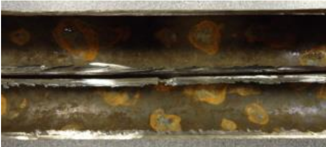
Figure 6. Attack on TP439 can be closely spaced multiple sites.
