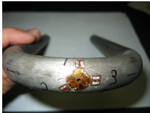
Figure 17. A u-bent tube containing a the drilled-hole strain gage method for determination of residual stresses
