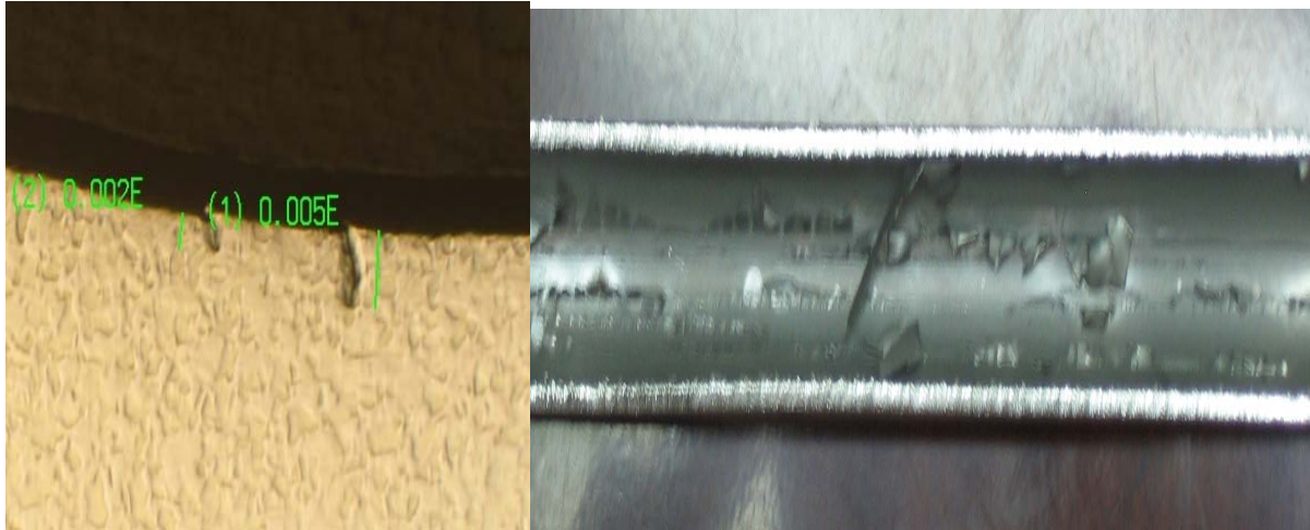
Figure 1 ID flaws in seamless tubing. The hollows made by the extrusion process are on the left and the rotary piercing process on the right.
