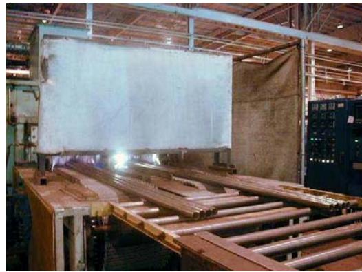
Figure 11 – Off-line furnace annealing of feedwater heater tubing
