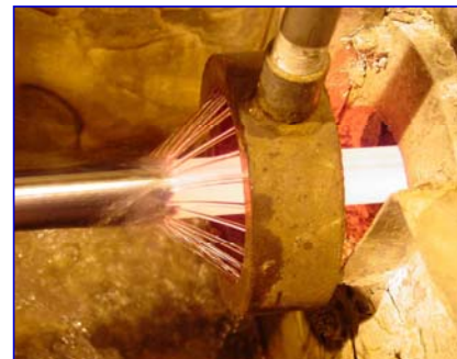
Figure 10 – In-line water quenching
