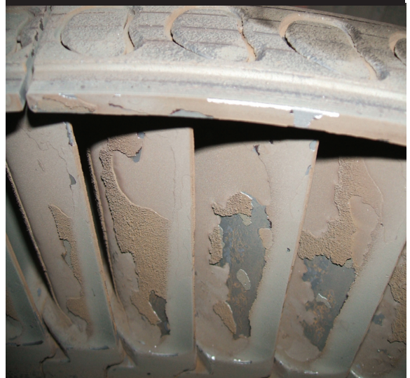
Copper deposits on a HP turbine. 2
