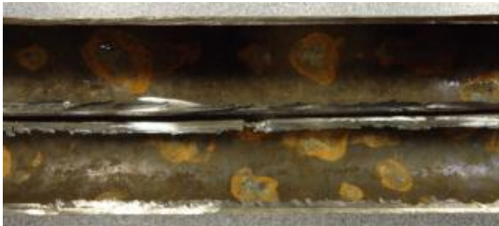
Figure 5 MIC attack of three different alloys – 90/10 Cu/Ni, Type 304 stainless steel, and Type 439 stainless steels. All of these occurred in less than 1 year after installation.
