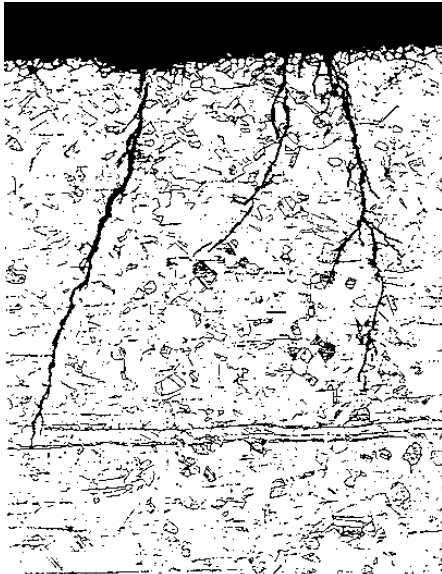
Figure 7 Transgranular Stress Corrosion Cracking in TP 304N Feedwater Heater Tubing
