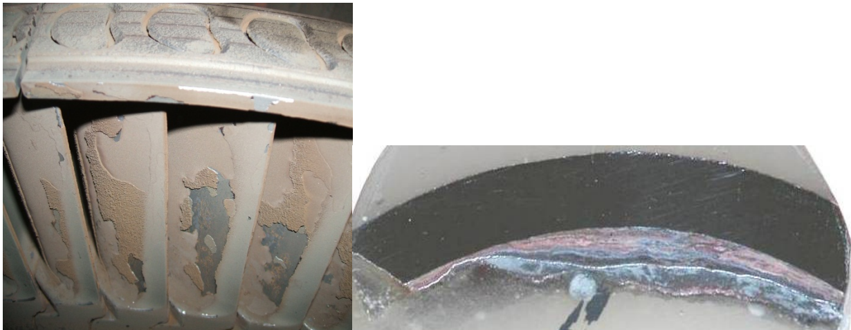
Figure 6. Copper deposits on HP turbine at Pacificorp Huntington Unit 2 and layered alternating iron and copper deposits on boiler tubes.(ref. 10)
