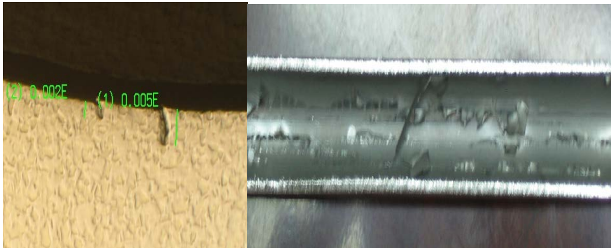
Figure 1 ID flaws in seamless stainless steel tubing. The hollows made by the extrusion process are on the left and the rotary piercing process on the right.
