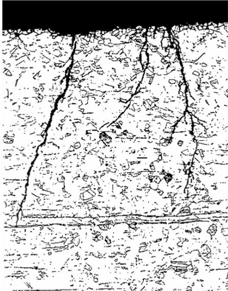
Figure 10 Chloride SCC of TP 304N
