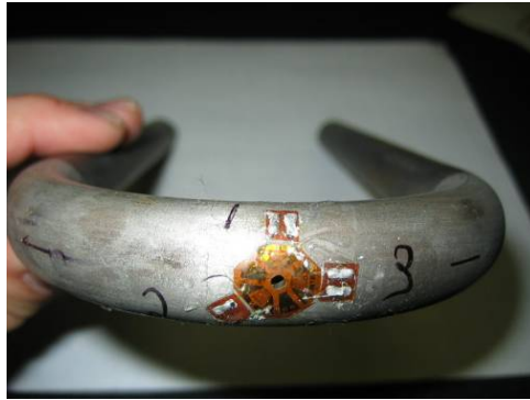
Figure 9. A u-bent tube containing a the drilled-hole strain gage method for determination of residual stresses
