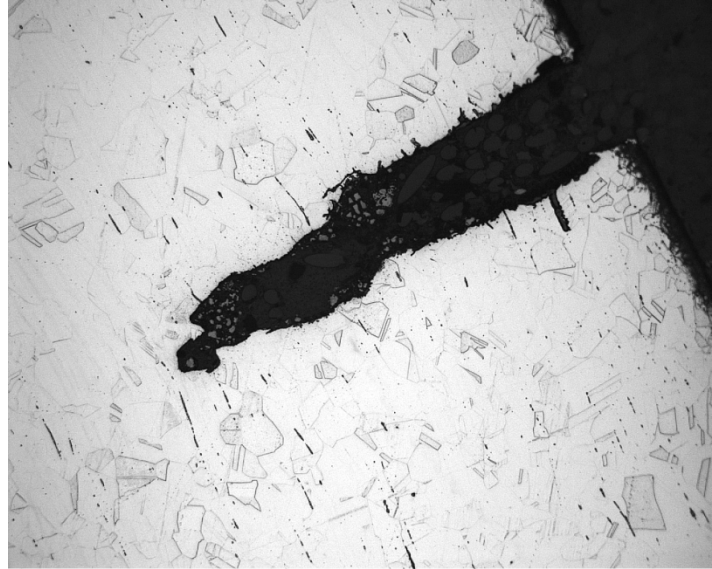
Figure 11 Thermal Fatigue Cracking of TP 304N
