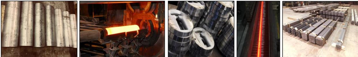
Figure 2. The titanium billets are subjected to beta heat treatment followed by extrusion using the required dies, thermally straightened, surface alpha case chemically removed and packed for shipment.
