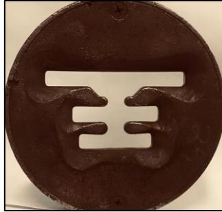
Figure 1. The profile of the die shown here provides the geometry of the shape to be extruded. Manufactured in-house from modified tool steel, the die is able to withstand intense heat and pressure generated during the extrusion process.
